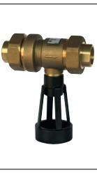
Designed to protect drinking water networks against fluids with risk up to category 3 according to NF EN1717. The device is designed to prevent any backflow that can be caused by back pressure or siphonage in the drinking water network.
