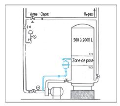
Installation on tank not provided with an opening in the connecting zone
