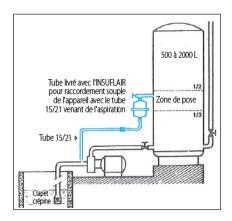
• Installation with tank fed from town water circuit
