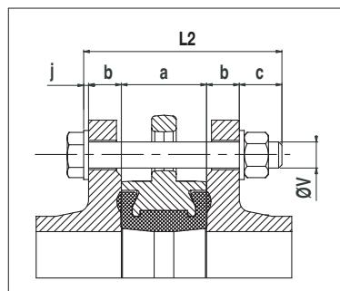
For wafer type and lugs with unthreaded holes ; assembly by bolts :
