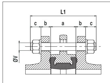
For wafer type and lugs with unthreaded holes ; assembly by rods :
