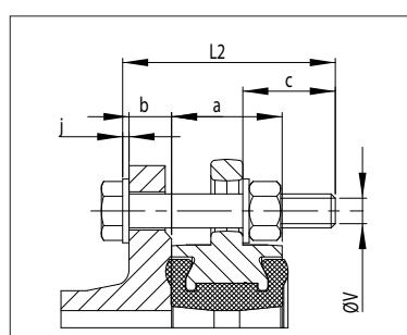
Version lug type with unthreaded holes, (permanent downstream dismantling) assembly by bolts :
