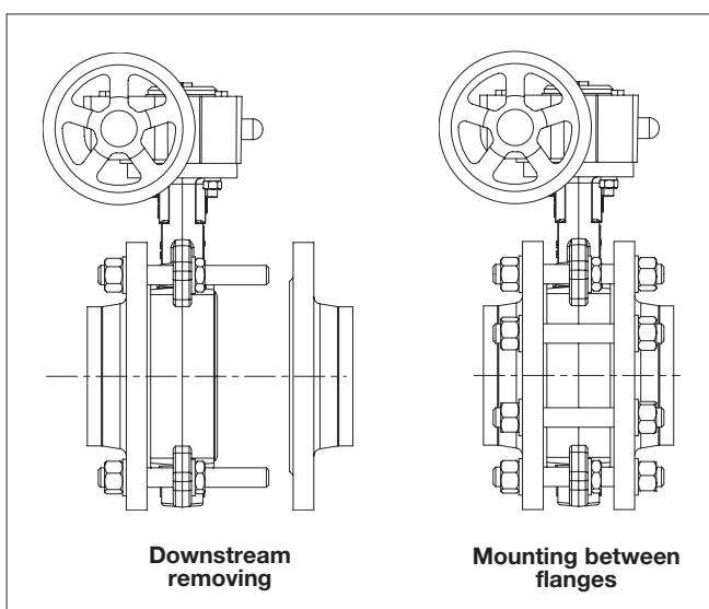
Use nuts with reduced face-to-face dimensions between the flange to be dismounted and the centering lugs.
