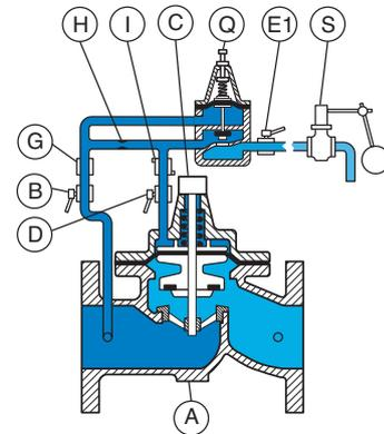
When the upstream pressure is getting higher than the preset pressure of pilot valve (Q), the pilot keeps open and allows the altitude regulation thanks to the pilot valve (S).
