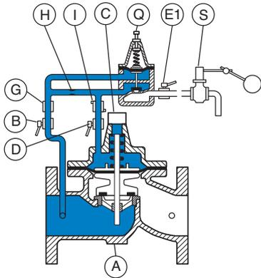
When upstream pressure is getting lower than the pressure required by the pilot (Q), the pilot will close and limit the flow circulation. The upstream pressure pushes on the membrane of the main valve (A) which closes. The upstream pressure increases and reaches the preset pressure of pilot (Q).
