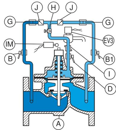
The pump stops, the solenoid valve (EV3) is switched off first. It put the upstream in communication with the upper chamber ; the valve begins slowly to close, slowed down by the needle valve (H).
