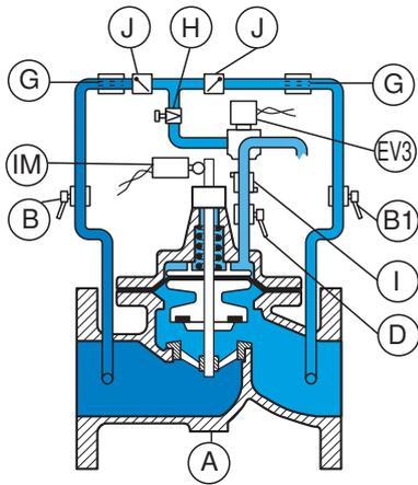
The pump starts, the valve is closed.
