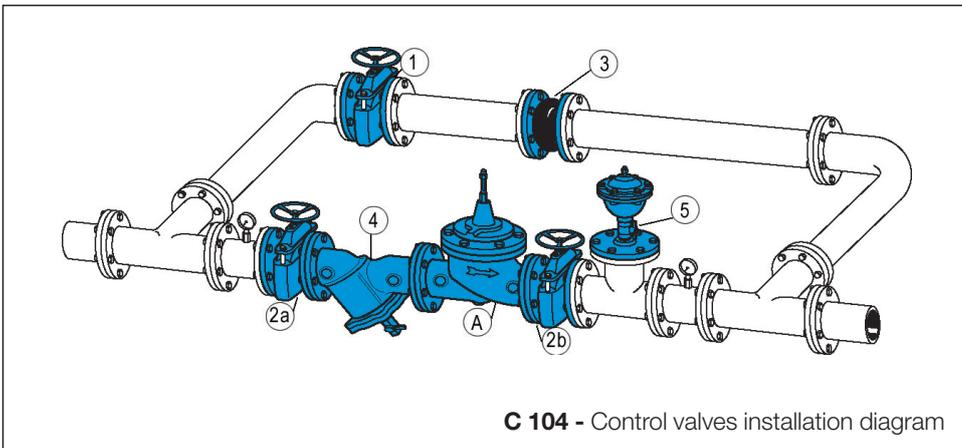
C 104 - Control valves installation diagram
