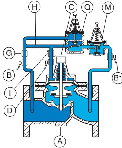
As soon as upstream pressure is getting higher than setting pressure of pilot (Q), pilot keeps open and allows downstream regulation thanks to pilot (M).
