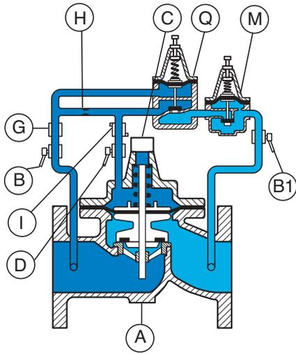
When upstream pressure is getting lower than the pressure required by the pilot (Q), the pilot will close and limit the flow circulation. The upstream pressure pushes on the membrane of the main valve (A) which closes. The upstream pressure increases and reaches the setting of pilot (Q).
