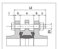
For wafer type and lugs with unthreaded holes type body; assembly by screws:
