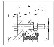
For lugs with unthreaded holes type body (permanent downstream dismantling); assembly by bolts:
