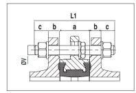
Mounting in case of downstream pipework dismantling (see page 13).
