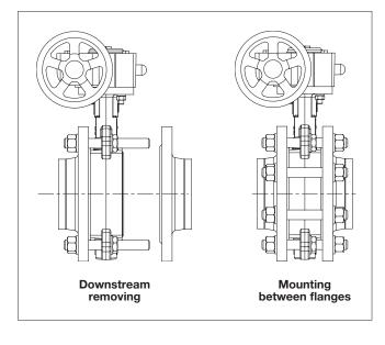
Use hexagon thin nuts between the flange to be dismounted and the centering lugs.
