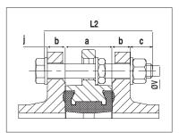
Mounting in case of downstream pipework dismantling (see page 13).
